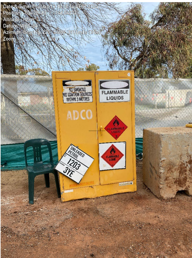
Bunded and signed Flammable Liquids cabinet.
