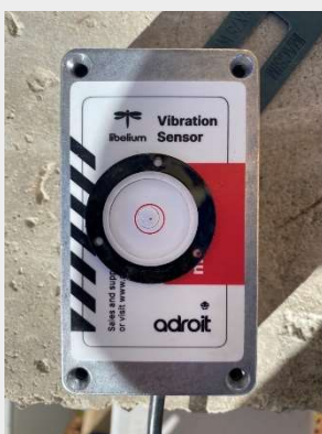
Fig 2 – The Vibration sensor is installed on a concrete block at the base of the permanent noise barrier near the imaging department. It needs to be installed level in all 3 planes (x, y, & z) to ensure that correct amplitude and velocity measurements will be recorded correctly.
