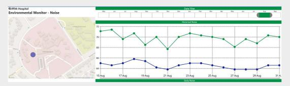
The noise readings from sensor NOISAU-009, located near the ADCO Site Sheds showed a peak noise value of 71.4 dB on  $16^{th}$  August 2023. This peak event lasted approximately 18 minutes.
