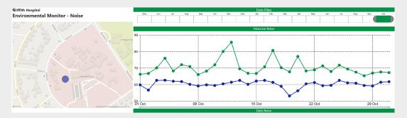
The noise readings from sensor NOISAU-009, located near the ADCO Site Sheds showed a peak noise value of 85.6dB on 12<sup>th</sup> October 2023. This peak event lasted approximately 18 minutes.
