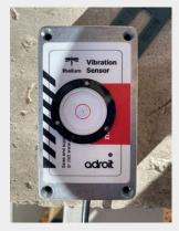
Fig 2 — The Vibration sensor is installed on a concrete block at the base of the permanent noise barrier near the imaging department. It needs to be installed level in all 3 planes (x, y, & z) to ensure that correct amplitude and velocity measurements will be recorded correctly.
