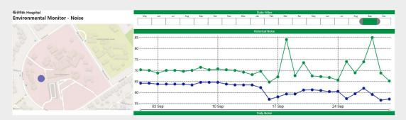
The noise readings from sensor NOISAU-009, located near the ADCO Site Sheds showed a peak noise value of 84.9dB on 28th September 2023. This peak event lasted approximately 18 minutes.
