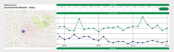
The noise readings from sensor NOISAU-009, located near the ADCO Site Sheds showed a peak noise value of 74.3dB on 18<sup>th</sup> July 2023. This peak event lasted approximately 18 minutes.
