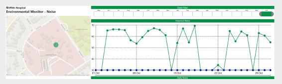
The noise readings from sensor NOISAU-005, located near the scanning department showed a peak noise value of 69.4dB on 18th October 2023.
