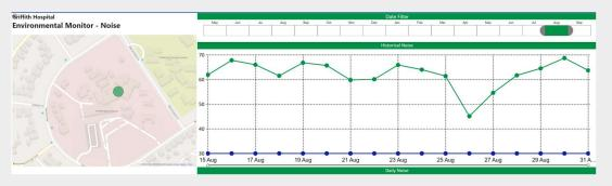
The noise readings from sensor NOISAU-005, located near the scanning department showed a peak noise value of 68.7dB on 30th August 2023.
