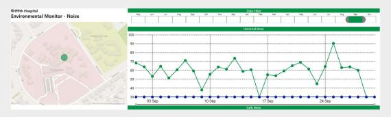
The noise readings from sensor NOISAU-005, located near the scanning department showed a peak noise value of 90.4dB on  $25^{th}$  September 2023.
